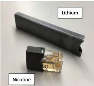
An e-cigarette showing the portions that contain the two hazards.
